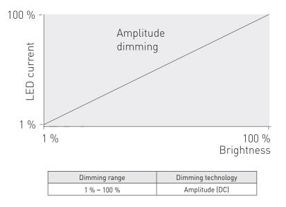
LC27MINI-DA-150-700 LED driver implements amplitude dimming technology across whole dimming range. Amplitude dimming offers the best available technology for dimming the light output in an accurate and flicker-free way to ensure high quality lighting in even the most demanding situations such as camera recording applications. Amplitude dimming technology complies with IEEE 1789-2015 recommendations of current modulation to mitigate health risks to viewers.
