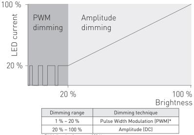
PWM dimming frequency 800 Hz
