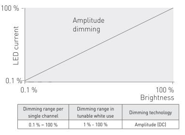
LL100iC-DA-100-800 LED driver implements amplitude dimming technology across whole dimming range. Amplitude dimming offers the best available technology for dimming the light output in an accurate and flicker-free way to ensure high quality lighting in even the most demanding situations such as camera recording applications. Amplitude dimming technology complies with IEEE 1789-2015 recommendations of current modulation to mitigate health risks to viewers.
