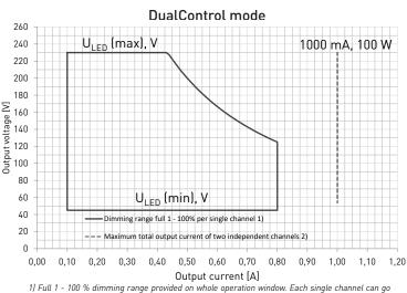
Full 1 - 100 % dimming range provided on whole operation window. Each single channel can go down to 1 % dimming at 100 - 800 mA.
