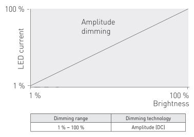
LL35HE-DA-80-400 LED driver implements amplitude dimming technology across whole dimming range. Amplitude dimming offers the best available technology for dimming the light output in an accurate and flicker-free way to ensure high quality lighting in even the most demanding situations such as camera recording applications. Amplitude dimming technology complies with IEEE 1789-2015 recommendations of current modulation to mitigate health risks to viewers.
