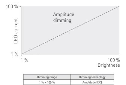
LC26MINI-DA-250-700 LED driver implements amplitude dimming technology across whole dimming range. Amplitude dimming offers the best available technology for dimming the light output in an accurate and flicker-free way to ensure high quality lighting in even the most demanding situations such as camera recording applications. Amplitude dimming technology complies with IEEE 1789-2015 recommendations of current modulation to mitigate health risks to viewers.
