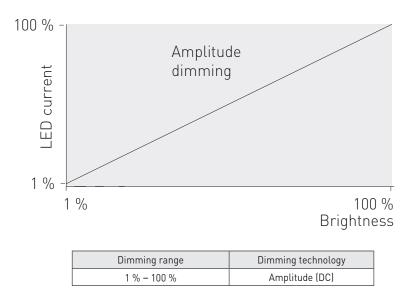
LC12TINY-DA-180-700 LED driver implements amplitude dimming technology across whole dimming range. Amplitude dimming offers the best available technology for dimming the light output in an accurate and flicker-free way to ensure high quality lighting in even the most demanding situations such as camera recording applications. Amplitude dimming technology complies with IEEE 1789-2015 recommendations of current modulation to mitigate health risks to viewers.
