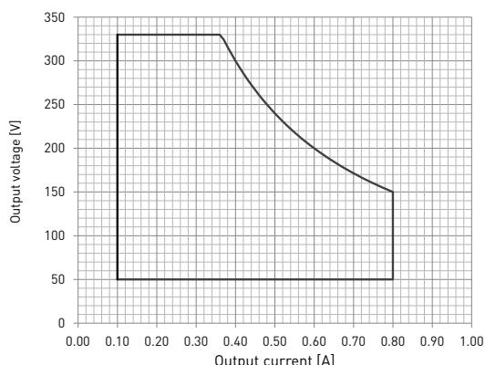
From 100 mA to 800 mA, full dimming range (1 % - 100 %) available in the whole area, restricted by the absolute minimum dimming current of 2 mA.
