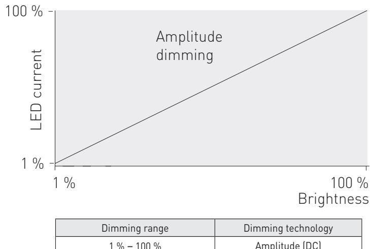
LL120HE-DA-100-800 LED driver implements amplitude dimming technology across whole dimming range. Amplitude dimming offers the best available technology for dimming the light output in an accurate and flicker-free way to ensure high quality lighting in even the most demanding situations such as camera recording applications. Amplitude dimming technology complies with IEEE 1789-2015 recommendations of current modulation to mitigate health risks to viewers.
