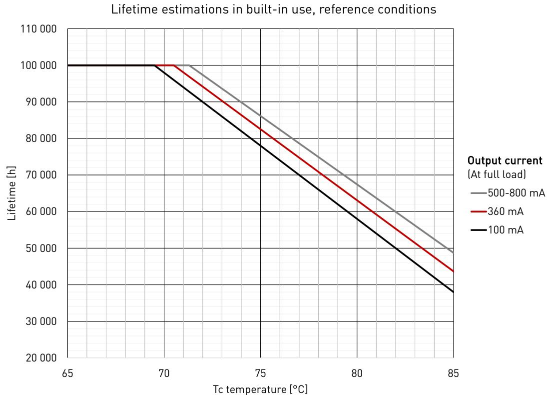
The shown  $t_c$  temperatures and lifetimes were measured in reference conditions i.e. metallic luminaire design and built-in use. Please refer to the used output current and  $t_c$  for the most accurate lifetime estimation.
