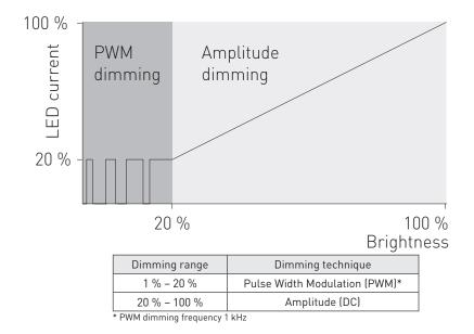
Helvar Components hybrid dimming products combine the best features from Amplitude dimming and from Pulse Width Modulation (PWM) dimming. CCR is a very efficient technique for dimming the light output especially on higher range. On lower range, the hybrid dimming products implement high-frequency PWM dimming to ensure high quality dimming from 20 % down to 1 % providing low flicker dimming performance.
