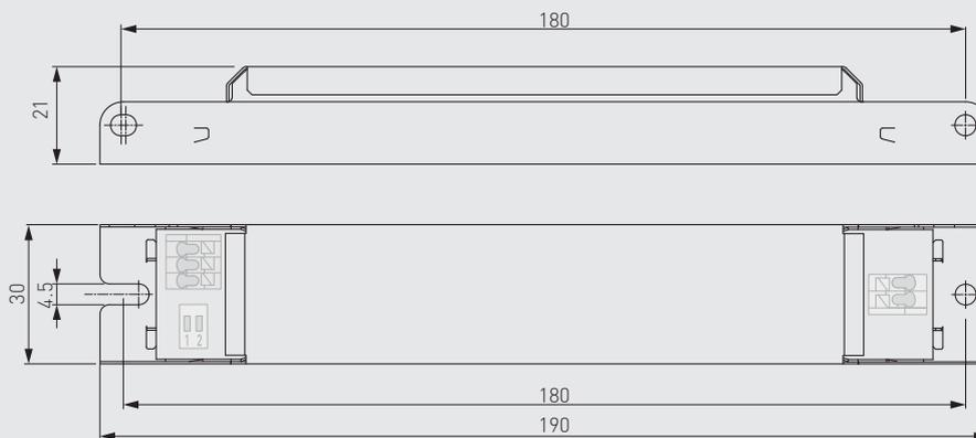
In LL18SEC-CC-200-350, the current can be set with dip-switches. With each combination of switch setup, a different output current value can be set. The maximum value can be reached with the dip-switch setting “11” (dip-switches pushed towards input connector) and minimum with setting “00” (pushed away from the input connector, see connections picture above). The output current values according to the dip-switch settings are presented below.
