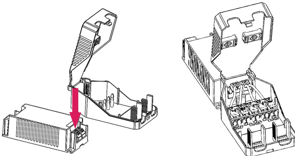
2. Connect L/N cables in on /off & Freedom models and L/N/DA1/DA2 cables in DALI models to the 5-place connector. Ensure that the cables are firmly and securely mounted into the connector!
