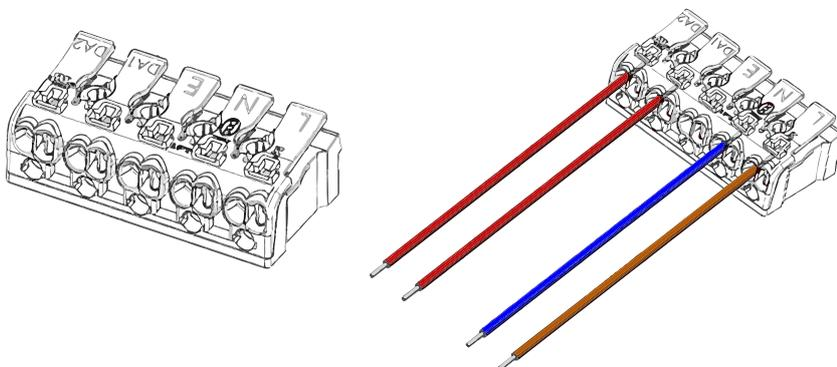
3. Connect the cables to the driver input into corresponding terminals. Ensure that the cables are firmly mounted.
