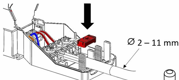
Ensure that cables are tightly locked.
