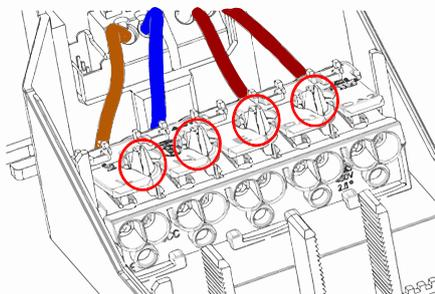
5. Connect wires into correct terminals according to driver datasheet instructions. Lock wires with the cable clamps by pressing them to place at the cable sheath.
