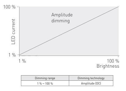
LC26MINI-DA-250-700-SR LED driver implements amplitude dimming technology across whole dimming range. Amplitude dimming offers the best available technology for dimming the light output in an accurate and flicker-free way to ensure high quality lighting in even the most demanding situations such as camera recording applications. Amplitude dimming technology complies with IEEE 1789-2015 recommendations of current modulation to mitigate health risks to viewers.
