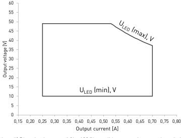
Note: 1) Dimming between 1 % - 100 % possible across the operating window, restricted by the absolute minimum dimming current of 7 mA.
