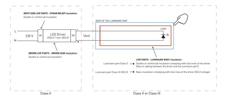
Note: The combination is Class II, even though Class III luminaire parts are used!
