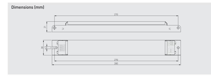
In LL150HE-CC-350-700-DS the current can be set with DIP switches. With each combination of switch setup, a different output current value can be set. The maximum value can be reached with the DIP switch setting "111" (DIP switches pushed towards label, see connections picture above) and minimum with all switches set to "0". The output current values according to the DIP switch settings are presented below.
