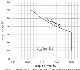
Note: Current value is adjustable in 50 mA steps via dip-switch. See dip-switch settings in page 3 for details.
