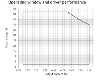
1) Dimming between 1 - 100 % possible accros the operating window, restricted by the absolute minimum dimming current of 3.5 mA 2) Current value is adjustable in steps via DIP switch. See DIP switch settings in page 5 for details.
