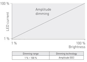
LC43MN22-DA-300-1050 LED driver implements amplitude dimming technology across whole dimming range. Amplitude dimming offers the best available technology for dimming the light output in an accurate and flicker-free way to ensure high quality lighting in even the most demanding situations such as camera recording applications. Amplitude dimming technology complies with IEEE 1789-2015 recommendations of current modulation to mitigate health risks to viewers.
