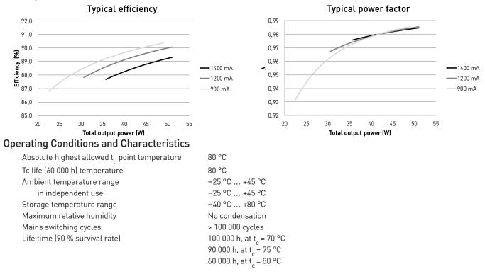
\*) For other than independent use, higher t<sub>a</sub> of the controlgear possible as long as highest allowed t<sub>c</sub> point temperature is not exceeded
