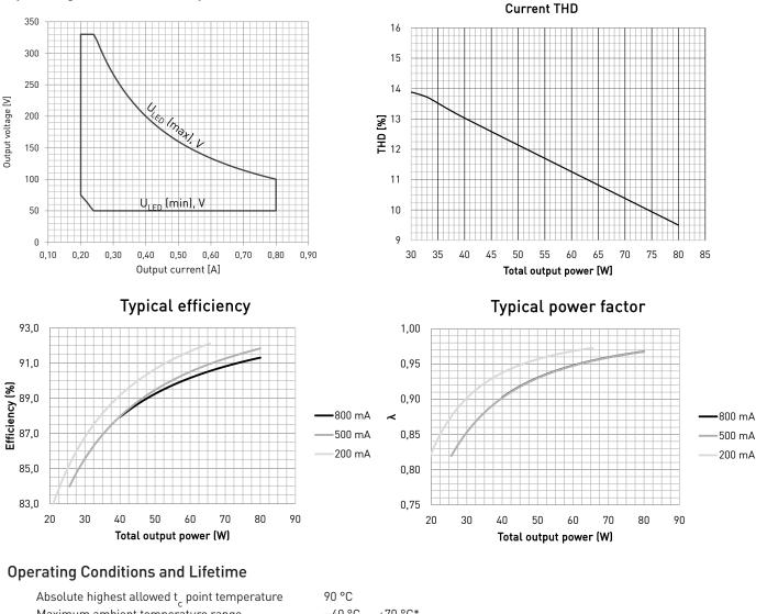
Maximum ambient temperature range Storage temperature range Maximum relative humidity -40 °C ... +70 °C\* -40 °C ... +80 °C No condensation
