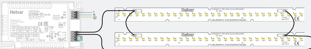
With LC35SE-CC-350-850 LED Driver, the selected output current is reached with 700 mA LED-Isset resistor (T90700, resistance value 7.15 kΩ)
