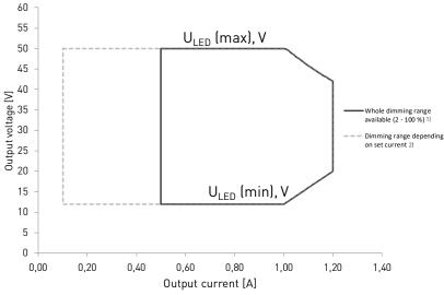
1) From 500 mA to 1200 mA, full dimming range ( 2 % - 100 %) and wide CCT dynamic range available in the whole area. Each single channel can dim down to 0.1 % level.
