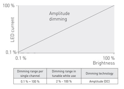
LL50iC-DA-100-1200 LED driver implements amplitude dimming technology across whole dimming range. Amplitude dimming offers the best available technology for dimming the light output in an accurate and flicker-free way to ensure high quality lighting in even the most demanding situations such as camera recording applications. Amplitude dimming technology complies with IEEE 1789-2015 recommendations of current modulation to mitigate health risks to viewers.
