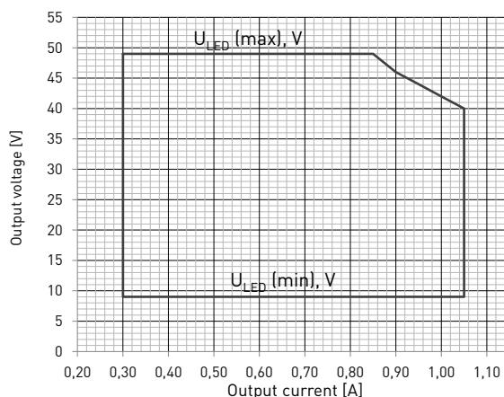
1) Dimming between 1 - 100 % possible across the operating window, restricted by the absolute minimum dimming current of 10 mA
