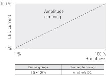
LL80HE-DA-100-800 LED driver implements amplitude dimming technology across whole dimming range. Amplitude dimming offers the best available technology for dimming the light output in an accurate and flicker-free way to ensure high quality lighting in even the most demanding situations such as camera recording applications. Amplitude dimming technology complies with IEEE 1789-2015 recommendations of current modulation to mitigate health risks to viewers.
