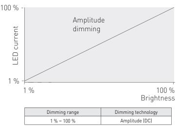
TR30-DA-350-700 LED driver implements amplitude dimming technology across whole dimming range. Amplitude dimming offers the best available technology for dimming the light output in an accurate and flicker-free way to ensure high quality lighting in even the most demanding situations such as camera recording applications. Amplitude dimming technology complies with IEEE 1789-2015 recommendations of current modulation to mitigate health risks to viewers.
