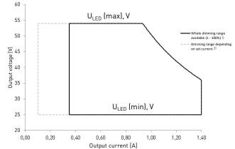
1) From 350 mA to 1400 mA, full dimming range (1 % - 100 %) available in the whole area. 2) From 100 mA to 350 mA, the absolute minimum dimming level is limited to 3.5 mA.
