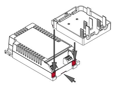
2. Connect wires into correct terminals according to driver datasheet instructions.
