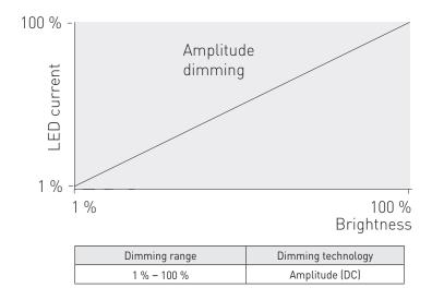
LC44SEC-DA-500-1000-LOOP LED driver implements amplitude dimming technology across whole dimming range. Amplitude dimming offers the best available technology for dimming the light output in an accurate and flicker-free way to ensure high quality lighting in even the most demanding situations such as camera recording applications. Amplitude dimming technology complies with IEEE 1789-2015 recommendations of current modulation to mitigate health risks to viewers.
