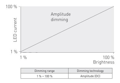
LC35SE-DA-350-850-LOOP LED driver implements amplitude dimming technology across whole dimming range. Amplitude dimming offers the best available technology for dimming the light output in an accurate and flicker-free way to ensure high quality lighting in even the most demanding situations such as camera recording applications. Amplitude dimming technology complies with IEEE 1789-2015 recommendations of current modulation to mitigate health risks to viewers.
