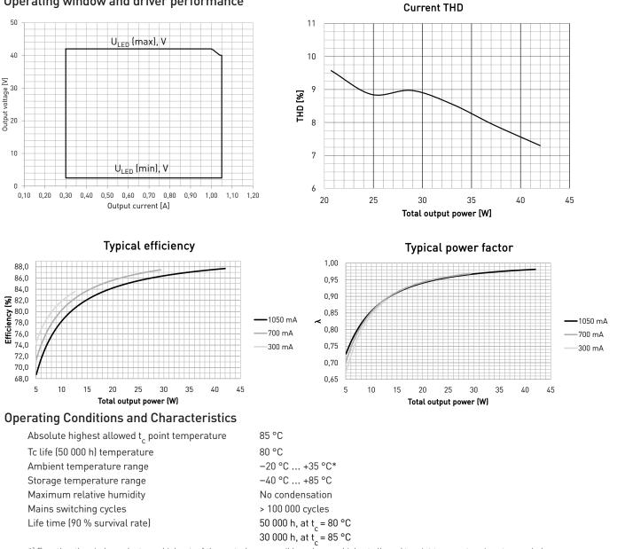
\*) For other than independent use, higher t, of the controlgear possible as long as highest allowed t, point temperature is not exceeded
