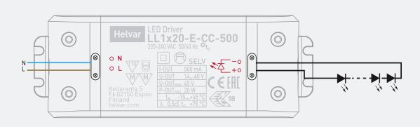
Note: Not suitable for load side switching operation.
