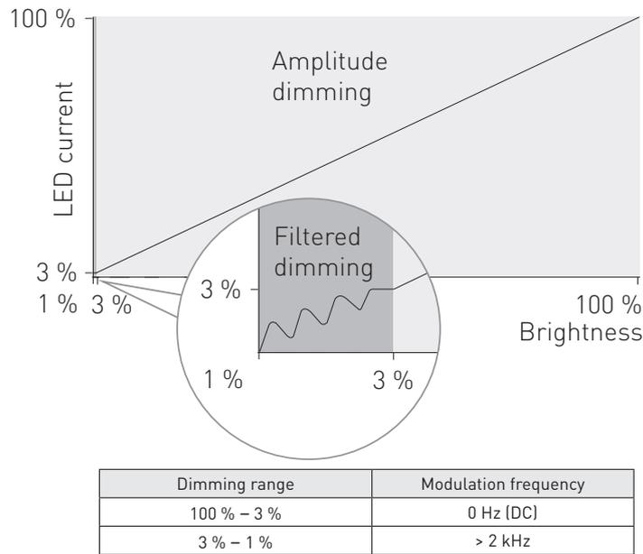
Filtered dimming technology is created to achieve extremely high quality and flicker free light output even at the lowest dimming levels. Light output is dimmed with amplitude dimming until the very lowest light levels (< 3%) and below that, stable light output is provided with filtered high frequency signal. Dimming technology complies with IEEE 1789-2015 recommendations of current modulation to mitigate health risks to viewers.
