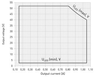
1) Dimming between 1 - 100 % possible accros the operating window, restricted by the absolute minimum dimming current of 3 mA 2) Current value is adjustable in steps via DIP switch. See DIP switch settings in page 3 for details.
