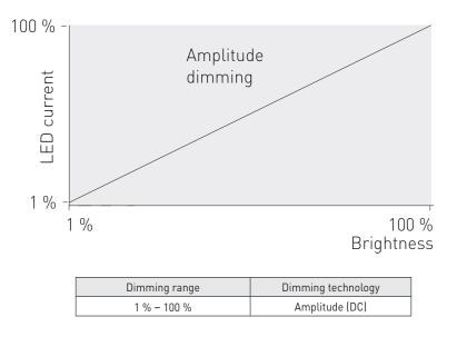
LC43MINI-DA-150-1050 LED driver implements amplitude dimming technology across whole dimming range. Amplitude dimming offers the best available technology for dimming the light output in an accurate and flicker-free way to ensure high quality lighting in even the most demanding situations such as camera recording applications. Amplitude dimming technology complies with IEEE 1789-2015 recommendations of current modulation to mitigate health risks to viewers.
