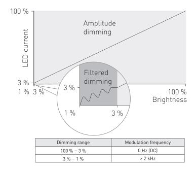
Filtered dimming technology is created to achieve extremely high quality and flicker free light output even at the lowest dimming levels. Light output is dimmed with amplitude dimming until the very lowest light levels (< 3%) and below that, stable light output is provided with filtered high frequency signal. Dimming technology complies with IEEE 1789-2015 recommendations of current modulation to mitigate health risks to viewers.
