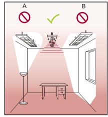
Do not place the sensor in direct line of artificial light sources, e.g. lamps or uplighters.
