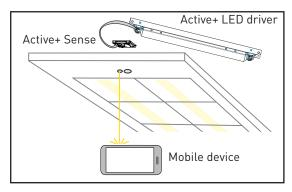
Note: Sensor holders are available to be used with the Active+ Sense: 5691 - ActiveAhead Sense Rectangular Sensor holder 5692 - ActiveAhead Sense Circular Sensor holder
