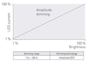
LL50SE-FD-100-1400 LED driver implements amplitude dimming technology across whole dimming range. Amplitude dimming offers the best available technology for dimming the light output in an accurate and flicker-free way to ensure high quality lighting in even the most demanding situations such as camera recording applications. Amplitude dimming technology complies with IEEE 1789-2015 recommendations of current modulation to mitigate health risks to viewers.
