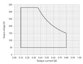
From 100 mA to 800 mA, full dimming range ( 1~% - 100~%) available in the whole area, restricted by the absolute minimum dimming current of 2~mA.
