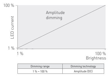
LL120HE-DA-100-800 LED driver implements amplitude dimming technology across whole dimming range. Amplitude dimming offers the best available technology for dimming the light output in an accurate and flicker-free way to ensure high quality lighting in even the most demanding situations such as camera recording applications. Amplitude dimming technology complies with IEEE 1789-2015 recommendations of current modulation to mitigate health risks to viewers.
