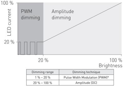
\* PWM dimming frequency 1 kHz
